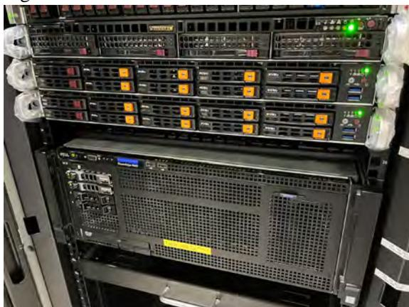
Fig. 2. High-performance computing machines: (top) the server for downloading diffraction images from the detector server, (2nd & 3rd) the image analysis server for diffraction scan, and (bottom) the detector server.
